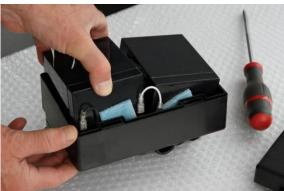
Use a small screwdriver to open the cover of the control box. Remove the batteries and unplug the connectors. Insert new batteries and reconnect them accordingly.
