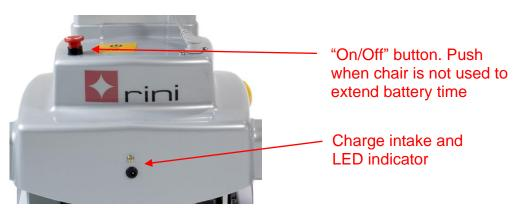
The "On/Off" button must be "On" during charging.
