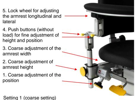
Move the position of the armrest by loosening the knob and sliding the armrests.
