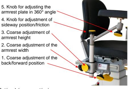
Setting 1 (coarse setting) Move the position of the armrest by loosening the knob and sliding the armrests.
